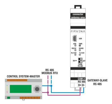
Note: If communication does not run on RS 232, RS 485, we recommend swapping the wires for RS 232 (Rx with Tx) or for RS 485 (D+ with D-) due to different specifications by control system manufacturers.
