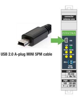
Note: For testing purposes and settings, the gateway can be powered via USB.
